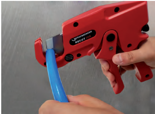
Cut the pipe with the special shear.
